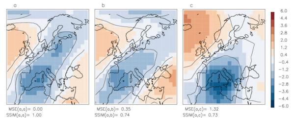
An example of pairs of images with similar MSE and different SSIM: both images b and c have similar MSE to the reference image a. But image b is structurally similar to a, c – dissimilar.
