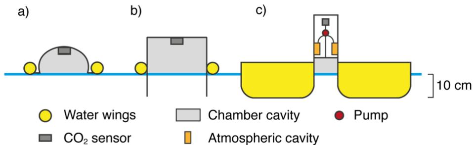
**Figure A2new: a) Classic floating chamber; b) Floating chamber with 10 cm long-edges; c) Platform design used in this study: 10 cm long-edges, rounded-edges, and flat and long water wings.**
