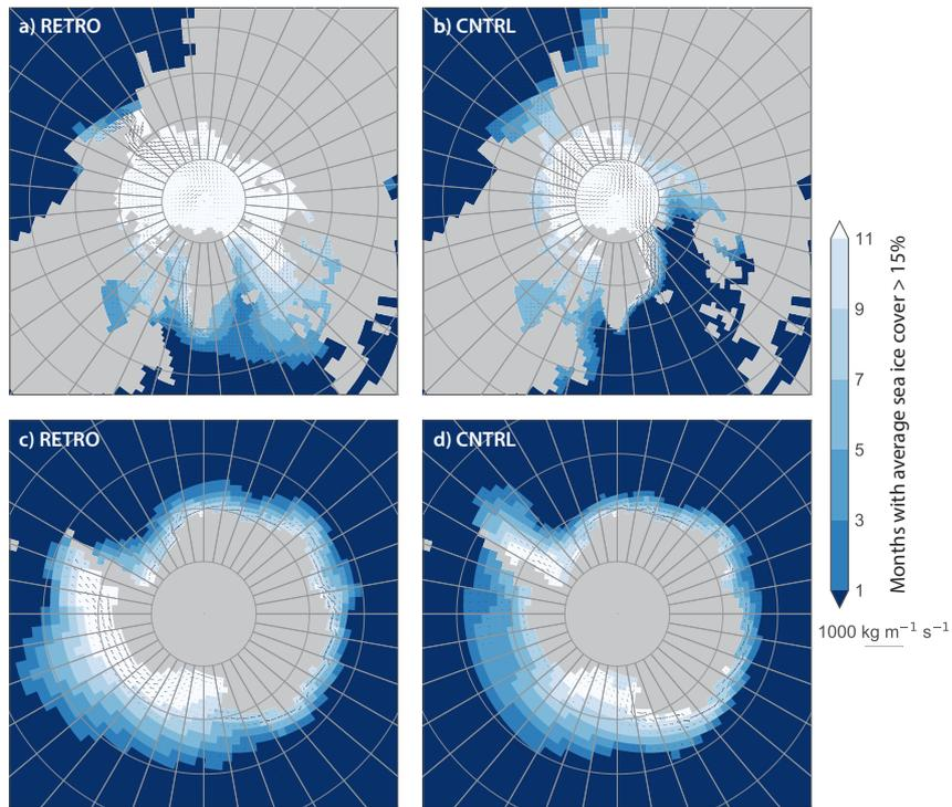
**Figure 3.** Duration of sea ice cover in RETRO (a, c) and CNTRL (b, d). The vectors show annual mean sea ice transport. For technical reasons no sea ice transport is displayed near the North Pole. The seasonal cycle of sea ice coverage is shown in a supplemental video.
