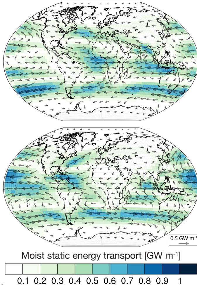
**Figure 5.** Moist static energy transport for RETRO (top) and CNTRL (bottom). To calculate the transports, we use 2 hourly data of velocities, surface pressure, temperature and specific humidity (Keith, 1995). The data are averaged over the last 100 years of the simulation.
