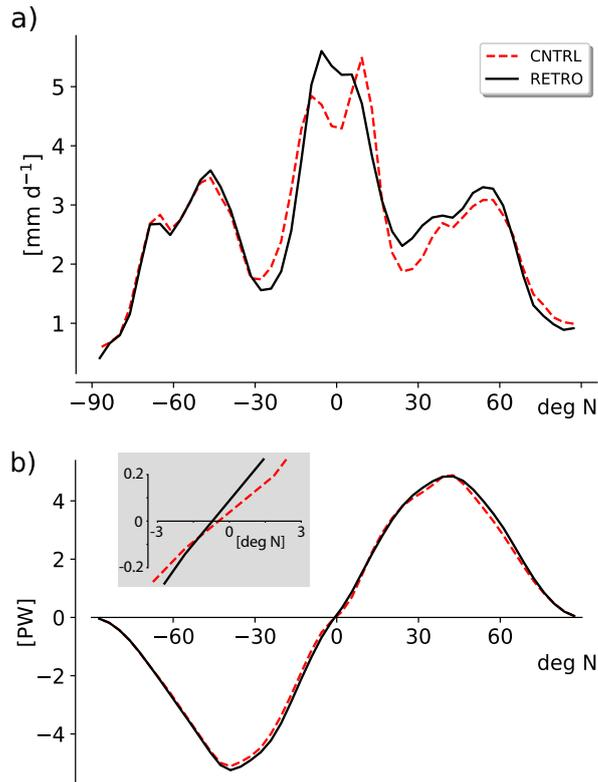
**Figure 7.** Zonally and annually averaged (a) precipitation; and (b) atmospheric energy flux for RETRO (black, solid) and CNTRL (red, dashed). The inset in panel (b) shows the atmospheric energy flux (computed as the integral of the vertical heat flux convergence as a function of latitude) in the vicinity of the zero crossing near the equator.
