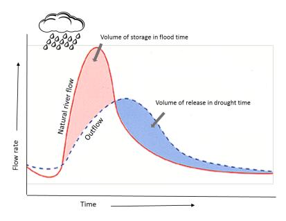
Figure 1: Human impact on hydrological extremes. Schematic example of the impact of dams and reservoirs, which tend to mitigate both hydrological extremes, i.e. lower flows during flood events and higher flows during drought conditions.
