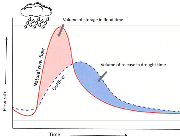
**Figure 1: Human impact on hydrological extremes. Schematic example of the impact of dams and reservoirs, which tend to mitigate both hydrological extremes, i.e. lower flows during flood events and higher flows during drought conditions.**
