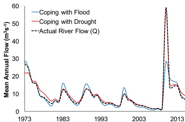
Figure 5: Example of modelling flood and drought in the Anthropocene. The diagram shows the result of a model run: actual river flows (black dash line) that result from changing norms in reservoir management between operation rules aiming to better cope with flood (blue line) and operation rules aiming to better cope with drought (red line).
