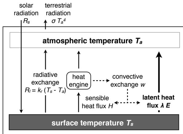
**Fig. 1.** Schematic illustration of the simple energy balance model that is used to describe the strength of the hydrologic cycle through the rate of surface evaporation,  $E$ , with the main variables and fluxes used here. After Kleidon and Renner (2013).
