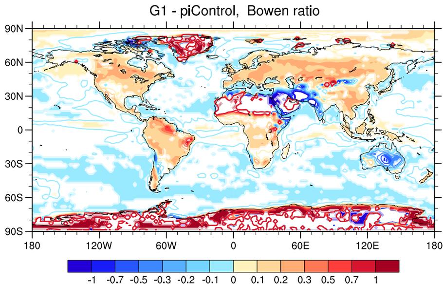
**Fig. 9.** Differences in Bowen ratio (ratio of surface sensible and latent heat fluxes) between the simulations G1 and piControl, averaged over the four ESMs. In regions with continuous color shading all models agree in the sign of the response.
