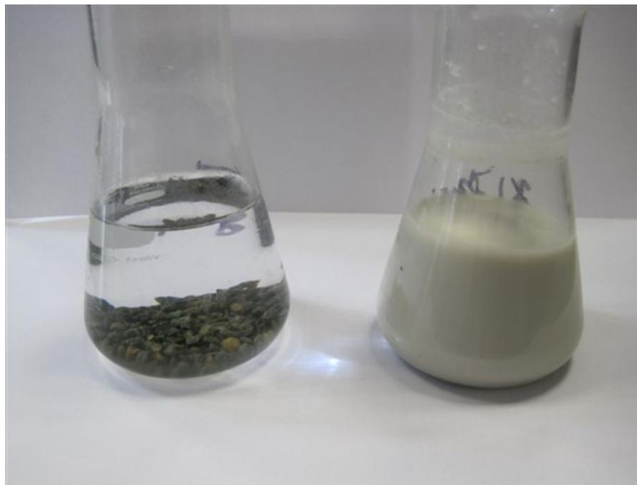
**Fig. 2.** Coarse (2–5 mm) olivine grains in clear water (left panel) give a white milky opaque suspension (right panel) after continuous motion on the table top rotary shaker during 10 days.
