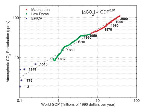
**Fig. A1.** Measured perturbations in atmospheric  ${\rm CO_2}$  concentrations from a baseline of 275 ppmv, compared with historical estimates of global GDP in inflation adjusted 1990 dollars, with associated year markers, and a linear fit to the data.
